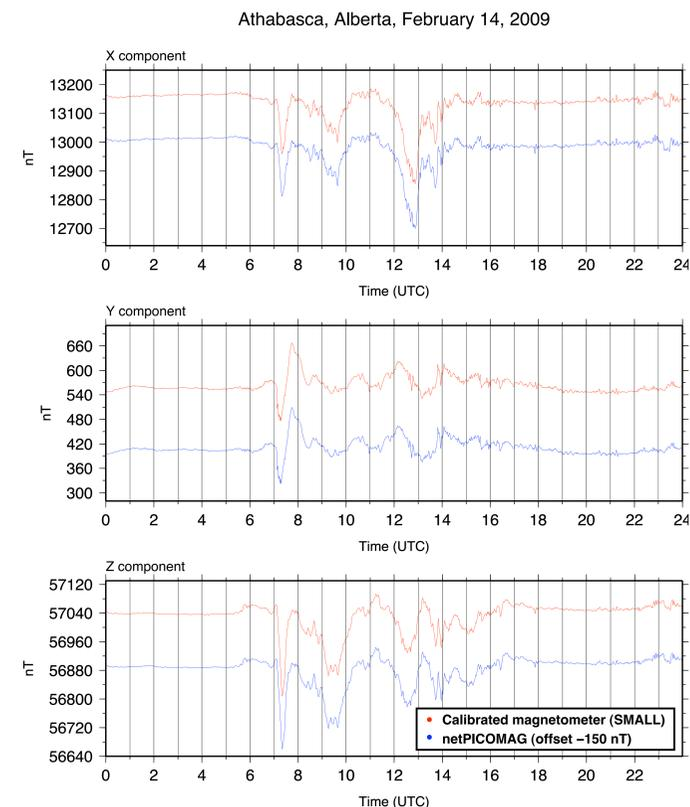
figure 3: Magnetic activity at Athabasca, Alberta on February 14, 2009. Data from a calibrated UCLA-SMALL fluxgate magnetometer (in red). NPM magnetic data (in blue) is offset by -150 nT.
