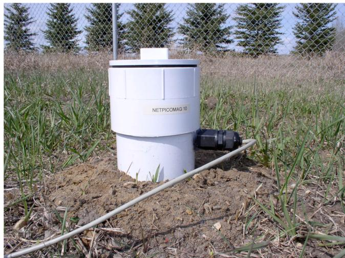
figure 1: NPM unit under test at Athabasca University Geophysical Observatory (AUGO), at Athabasca, Alberta.
